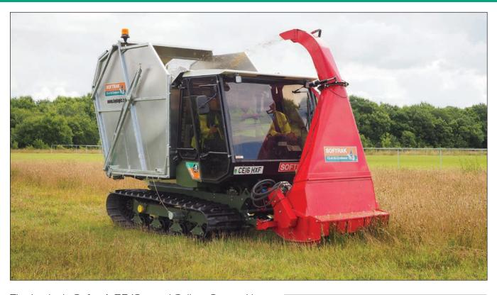
The Loglogic **Softrak** 75 'Cut and Collect System' is a purpose built low ground pressure vehicle, fitted with a front mounted flail harvester, for use in the restoration and harvesting of all types of vegetation. On wetland habitats its extremely low ground pressure and unique flexible rubber track ensures minimal damage to both flora and fauna in these environmentally sensitive areas.
