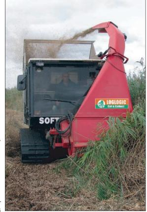
The chopped material is blown over the cab into a Front loading, 8 m3 rear bulk bin comprising of a lightweight galvanised steel frame and aluminium clad container with a full height automatic opening/closing door.
