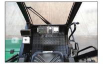
The comfortable cab comes with rubber suspension, tinted glass, full height door, opening side window and soundproofing as standard. With a full heating and ventilation system (optional air conditioning) and dust filtration stress free operation is ensured in all conditions. "Margard" polycarbonate front and rear safety screens with a silicone scratch resistant coating are fitted as standard. The cab is fitted as standard with a heavy-duty suspension seat and lap belt.
