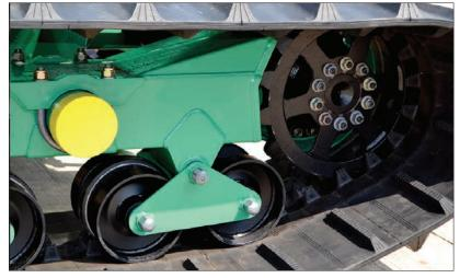
tend to ride over undulations in the ground, rather than shearing off the vegetation when turning. The cleat height can be reduced on request where high traction is not an issue.
