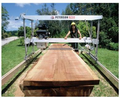
You no longer need to slab defects either, as you can easily dimensional-saw around them, getting the most value out of your log.
